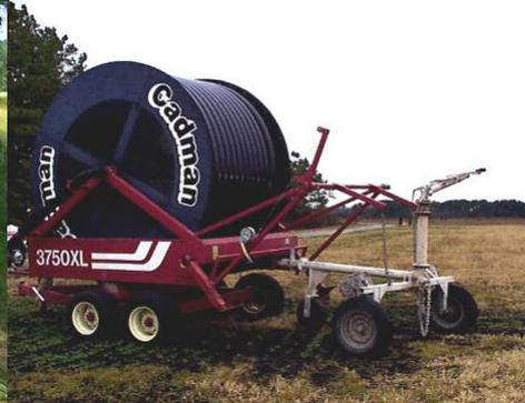
Hose reel pull irrigation systems are used in many field nurseries, however they require as much as 350 gallons of water per minute to operate. During droughts, irrigation supplies are often limited and adequate irrigation supplies are not available. In addition, these irrigation systems wet all soil surfaces in the field, therefore weed seeds germinate ready increasing weed pressure and weed management practices.
