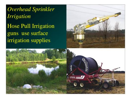
Hose reel pull irrigation systems are used in many field nurseries, however they require as much as 350 gallons of water per minute to operate. During droughts, irrigation supplies are often limited and adequate irrigation supplies are not available. In addition, these irrigation systems wet all soil surfaces in the field, therefore weed seeds germinate ready increasing weed pressure and weed management practices.
