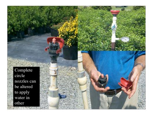
A variety of overhead sprinkler nozzles types are available. In this slide, the rotation pattern of the nozzle can be adjusted to cover a particular area. However, water volume applied is not adjustable, therefore, irrigation application is not as uniform as impact sprinklers designed to cover specific areas.
