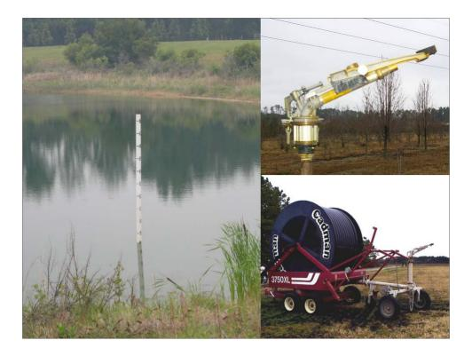
Large hose pull and over head gun irrigation systems require a power source and pump that can supply as much as 250 gallons per minute at 80 psi for overhead irrigation of nursery fields. The entire field is irrigated as compared to drip irrigation which only applies water down crop rows.
