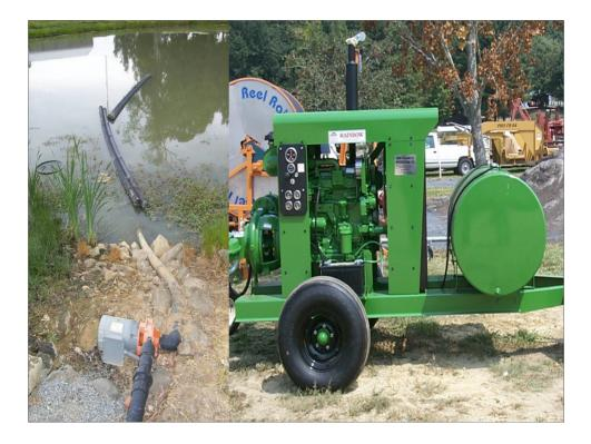
Electricity may or may not be available at field nursery sites. Drip irrigation systems only require small motors and low volume pumps as seen on the left of this slide, therefore availability for electrical service is preferred. In comparison, over head hose real and gun systems are often powered by large diesel motor driven pumps and can be operated in remote areas without electrical service.
