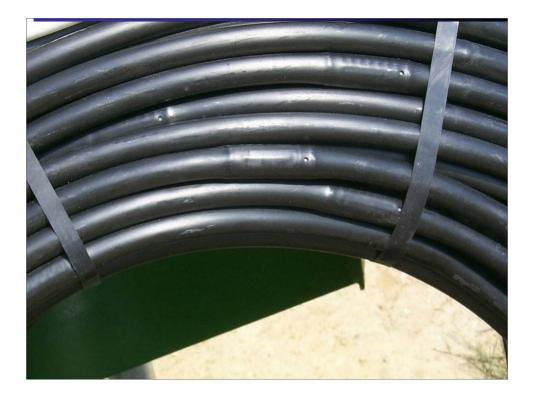
In line drip irrigation emitter tubing has become a standard for field production since labor for installation of drip buttons is no longer required. In line emitter drip tube can be purchased with various spacing of emitters such as 12, 18 or 24 inch spacing between emitters and flow rates from ½ gallon per hour to 5 gallons per hour, based upon spacing of nursery crops and soil infiltration rates.
