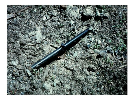
Buttons or spray emitters installed in drip tube requires considerable labor and may prove to be more expensive and less convenient than buying irrigation tubing with factory installed emitters.
