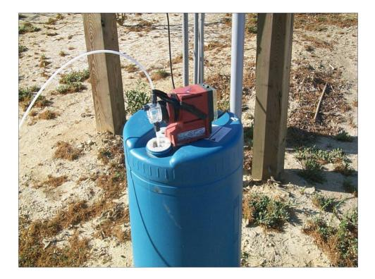
A liquid fertilizer stock tank and injector can be installed for application of fertilizer via the drip irrigation system.
