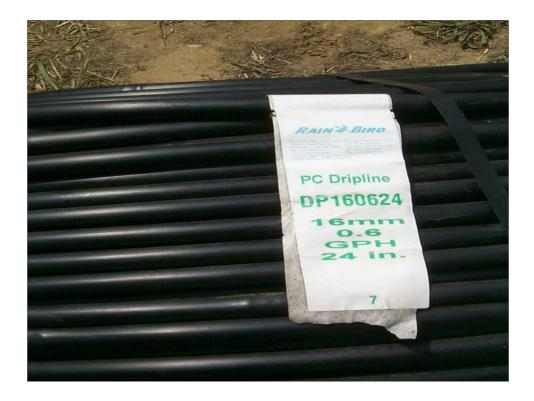
Drip tubing shown in this picture applies 0.6 gallons per hour. Emitters are spaced at 24 inches along the drip tubing.
